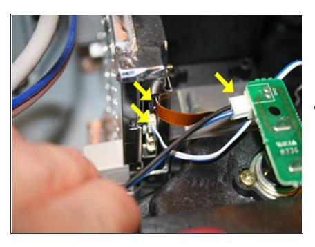
Remove the bad color wheel. The color wheel is held in place with three screws. Remove the screws and the color wheel. The color wheel may be stuck in place with the foam tape, but that'll give with a small tug. To remove the wheel cleanly, I lifted the front edge and slid it toward the front.
