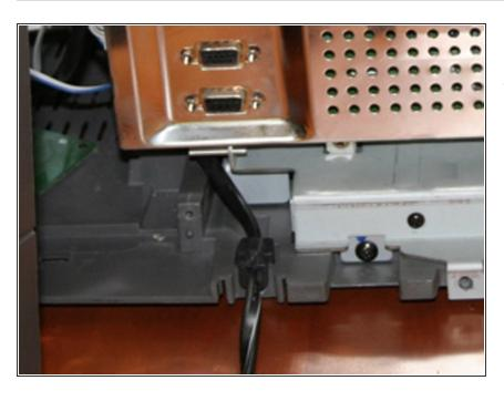
Carefully note how the power cable is positioned in the set, and the route it takes out the back. Once you have done that, pull the power cord out of it's notch in the bottom of the case. It's blocking the next part that has to slide out.
