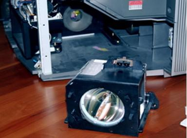
Remove the projector lamp. This may be unnecessary, but (a) it let's you see your target (the color wheel) and (b) it just seems like the safe thing to do. It's easy. Just unscrew the two brass screws holding it in. It's on the right side of the TV. The screws won't come out, just pull them out with the whole unit by pulling on the handle and sliding it straight out. Carefully store it somewhere safe.
