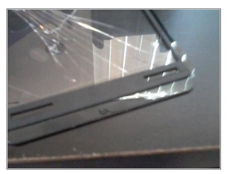
remove the rubber on the back of digitizer and transfer it over to the new digitizer make sure to use a heat gun to eat the adhesive on the backside of rubber to get off easily
