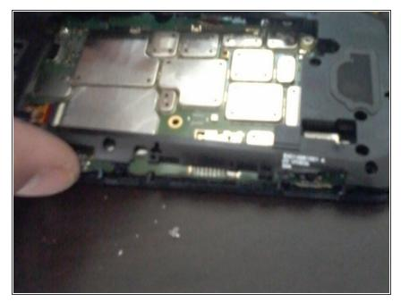
Now remove the circuit board's protective cover (the one you just unscrewed) by lifting it gently from the top. Three tabs need to be unclipped using the pry tool. Unclip at least 2 of the 3 clips and final tab should loosen on its own.
