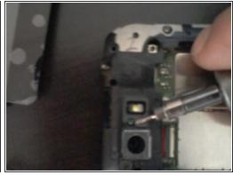
Remove the black screws around the outer edges and the 4 silver screws. (You'll find a silver screw on each side of the vibrator motor and on each side of the rear camera.)
