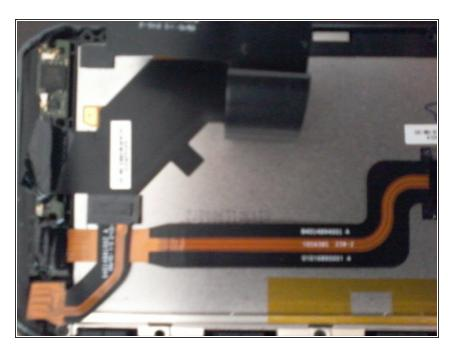
remove the 3 screws that hold the top circuit board to the phone
