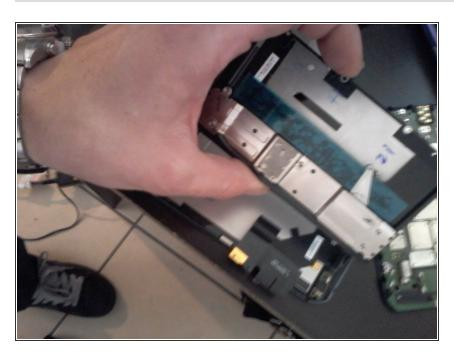
remove the back plate to the LCD screen being careful not to tear the ribbon cables and slide them through the slot.. then set it aside
