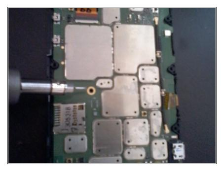
remove the one silver screw in the center of the circuit board which is holding it down
