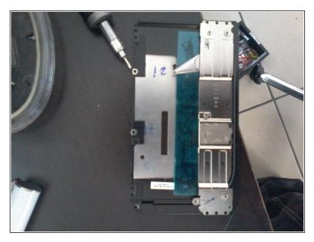
Remove the 7 screws ont the outer edge of the back lcd display
