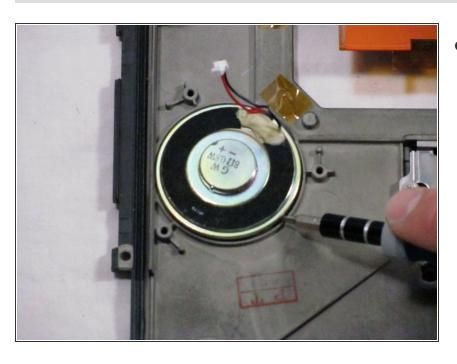
Pry out the speaker using a flat screw driver or a blue pry tool. It is held in with an adhesive.
