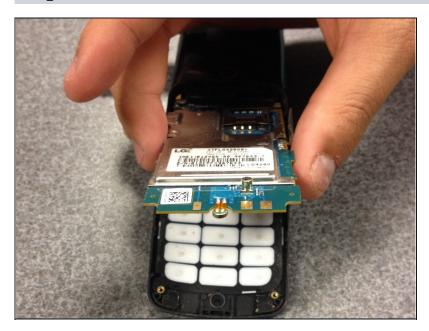
• Remove the layer connected with the keypad.
