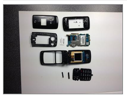
Remove all loose part, and should result in the components shown in the picture.
