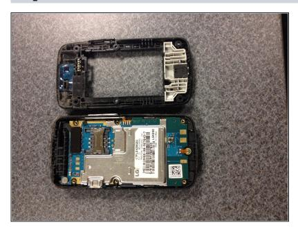
Remove the back part of the phone to expose the layers inside.
