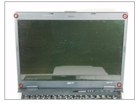
Pry out the 4 screw covers with a dental pick or other small pointed tool, and remove the screws located beneath them.
