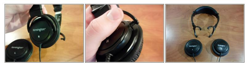
• Repeat the process in Step 1 to remove the right speaker clamp.
