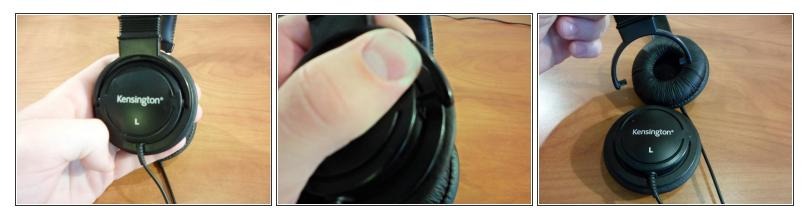
• Starting with the left speaker first, pull out one side of the speaker clamp where the clamp enters the hole on the speaker cover.
