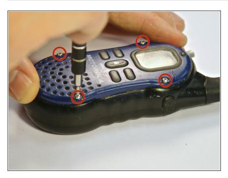
Remove the four 3 millimeter T6
