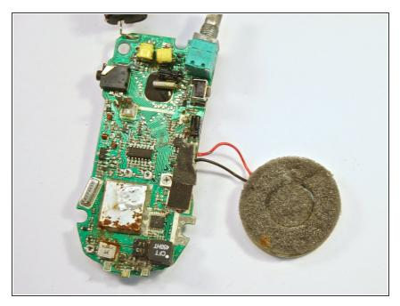
After pulling the circuit board away from the backplate, the result should be as shown in the picture.
