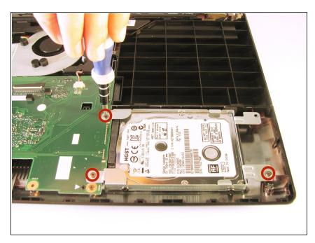
Unscrew the three 5.5 mm Phillips #0 screws with the Phillips #0 Screwdriver.
