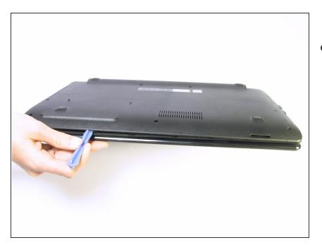
Use the plastic opening tool to separate the keyboard plate cover from the bottom cover. In order to do this, insert the plastic opening tool in between the keyboard plate cover and the bottom cover, then slide along edges to pry open.
