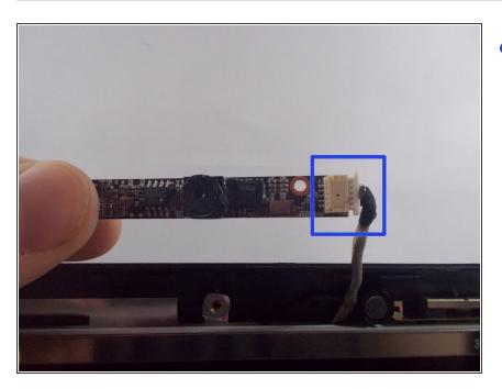
Disconnect the cable on the right side of the camera board by pulling firmly on the connector.
