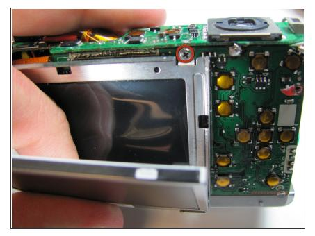
• Remove the screw underneath LCD screen with the Phillips #00. The screw measures 4.1mm in length.
