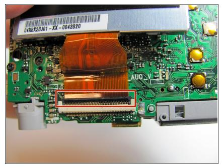
• Flip up the black tab on the bottom of the LCD screen with a fingertip.
