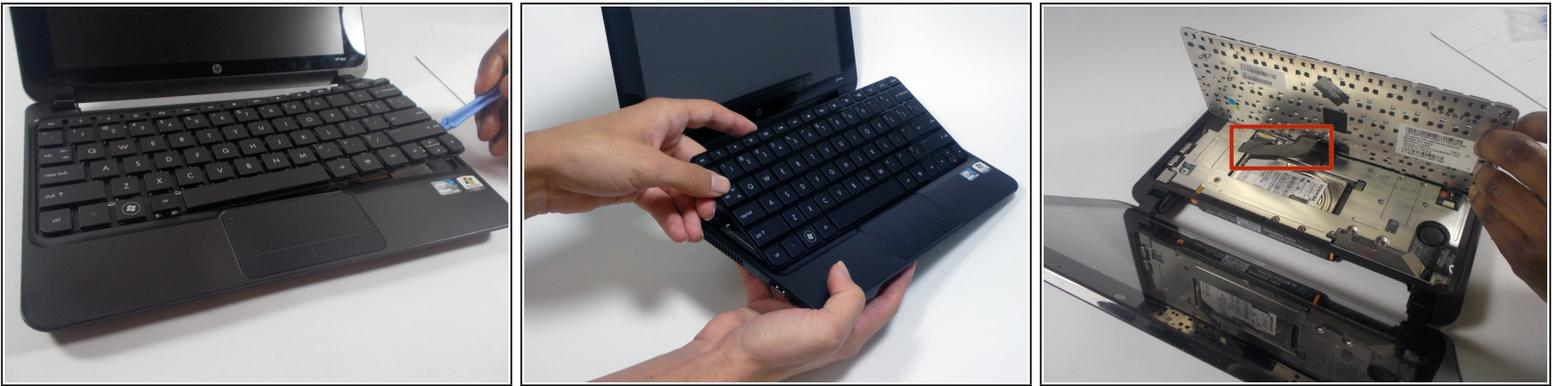
**i** After removing the plastic casing surrounding the keys, carefully lift the full keyboard from the netbook using a plastic opening tool.
