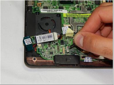
Detach the Bluetooth wire located below the fan by gently pulling it upward.
