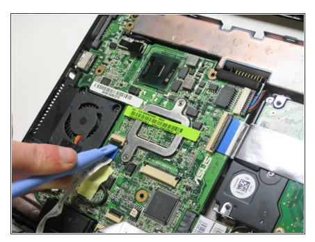
Detach the track pad ribbon by using a plastic opening tool to raise up the black pad.
