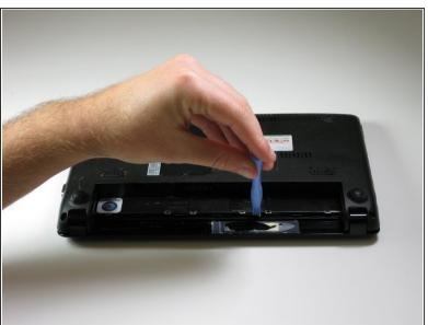
Use a plastic opening tool to pull up the four metal latches in the battery cavity that is located on the bottom of the laptop.
