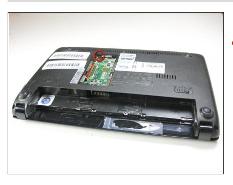
Use a Phillips #1 screwdriver to remove one 6.5 mm screw located next to the RAM.
