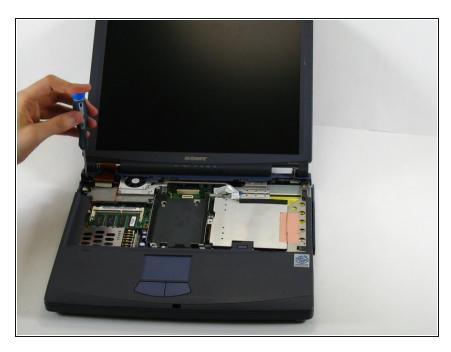
Remove the screw in the upper left corner that connects the display frame to the laptop.
