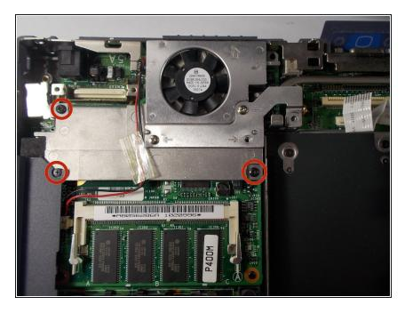
Remove the three black screws with the #00 Philips head screw driver.
