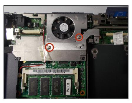
Remove the two silver screws with a #00 Philips head screw driver.
