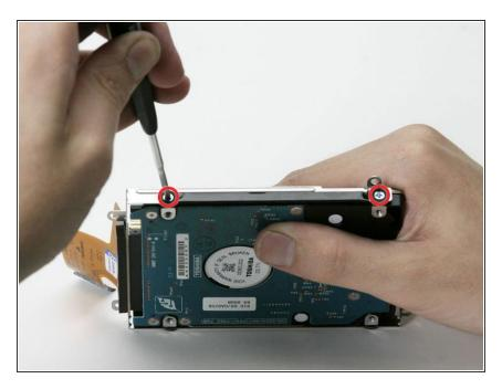
• Remove the two silver Phillips screws from either side of the hard drive (four screws total).
