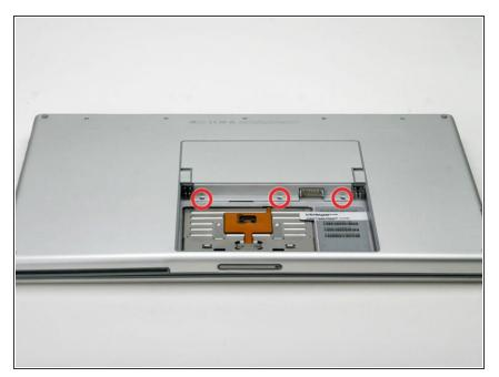
• Remove the three identical Phillips screws from the memory door.
