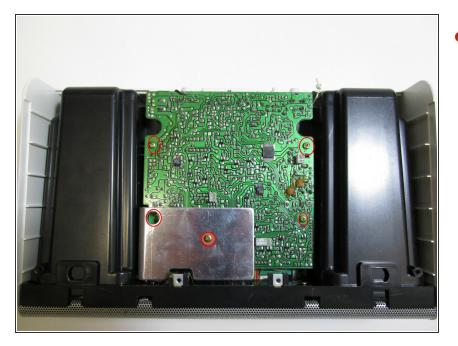
Remove the 5 screws with a #2 Phillips screwdriver.
