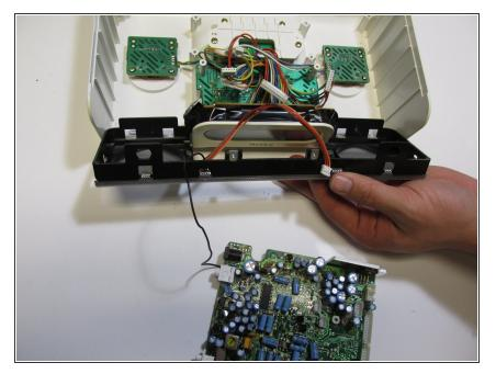
Remove the front piece by pulling up until it hits the plastic pieces sticking out from the display screen. Then pull it out horizontally from the device.
