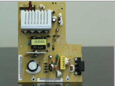
Lift the power supply out of the unit.
