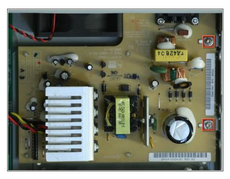
Rotate the device 180 degrees and remove the two T10 screws from the power supply board.
