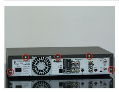
Remove the five T10 screws from the rear of the case using the Torx screwdriver.
