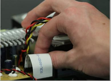
Carefully remove the ribbon cable from the power supply. Hold the ribbon on both sides and pull
