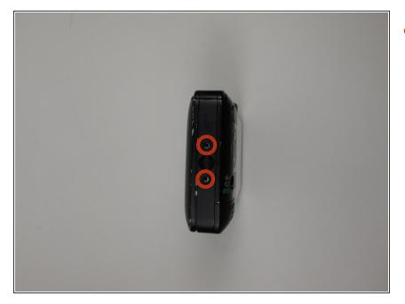
• There are 2 screws located on the left side of the camera. These screw locations are depicted with the red circle markings in the photos. These screws are 2.0 mm long.
