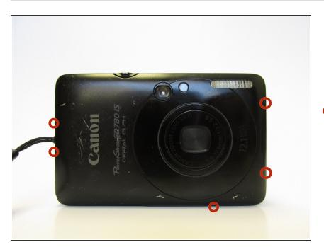
After the battery is removed, use a screwdriver to remove the five outermost screws on the camera to allow for a case replacement. Keep in mind that keeping track of where each screw came from is crucial for when putting the camera back together.
