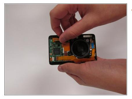
Remove the front panel of the camera case to expose the top left copper strip. Gently pull upward on the strip to disconnect it from the camera.
