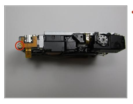
Using a screwdriver, remove the screw that attaches the charging mechanism to the body of the camera. This will allow the mechanism to be released from the camera.
