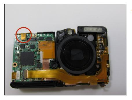
Once you remove the back portion of the camera, you will see the charging component. Remove the metallic strip on the charging component which attaches it to the motherboard.
