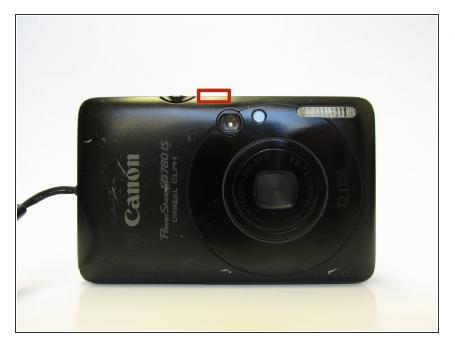
Begin by turning off the camera and removing the battery to avoid any shock injuries.
