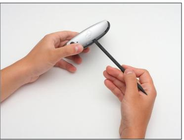
• Using a spudger, gently pry apart the back case from the front case. It is easier to start on a side and work your way around the device.
