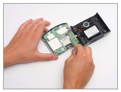
Once the two covers are separated, use tweezers, or even your fingers, to gently disconnect the two sets of wires that are connected to the motherboard from the back cover. You may have to wiggle the wires a little bit to get them to disconnect.
