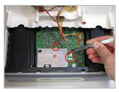
Use tweezers to unplug the three wires connected to the circuit board.
