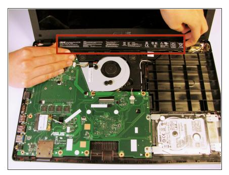
Remove the battery from the laptop by applying pressure on both ends and lifting it out of the case.
