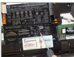
Using a screwdriver, remove the three 6.6 mm screws highlighted with the red circles in the first picture above.
