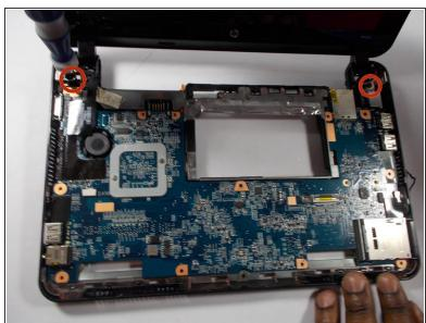
Use a screwdriver to remove the 9.3 mm screws on top of the motherboard.
