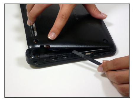
from the netbook easily, use the spudger to pry off the back case by the edge near the battery compartment, and work your way to the sides. The case will then pivot along the front edge.
