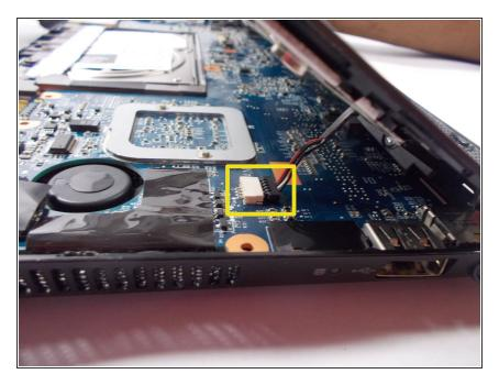
Locate the cable that connects the trackpad to the motherboard and carefully remove it.
