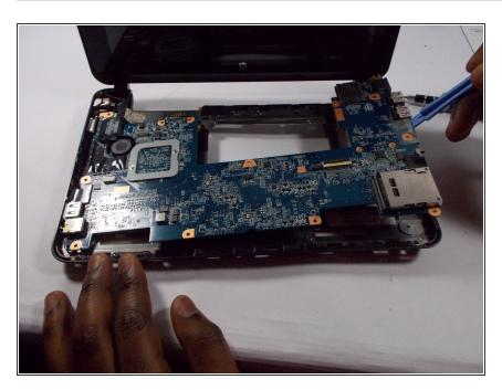
Use a spudger to carefully remove the motherboard.
