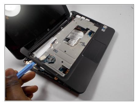
Use the spudger to peel the front black plastic plate from the rest of the case, starting at a corner and working your way around the entire case.
