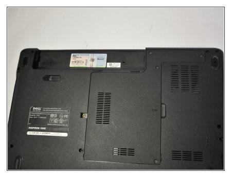
• Slide the battery out of the battery bay.
