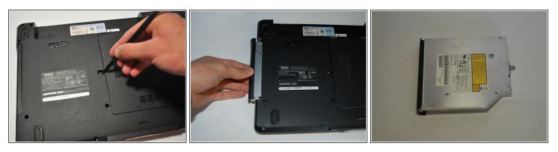
• Push the Optical Disk Drive out using a spudger tool as shown and pull from the front cover of the Optical Disk Drive.
