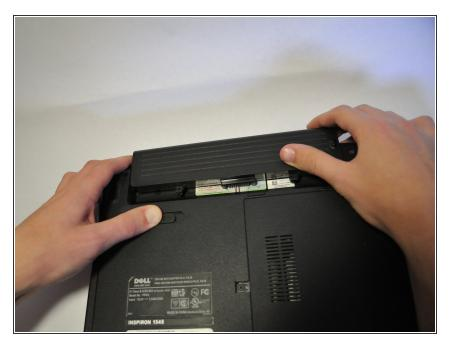
Slide the release latch while simultaneously pulling backwards on the battery.
