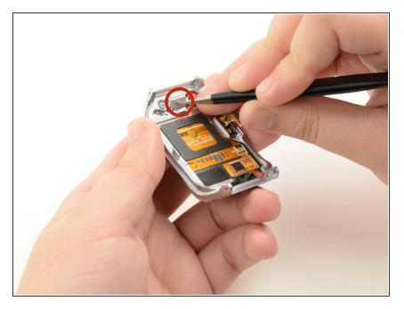
Use either the tweezers or the spudger to push the button peg out through the hole.
