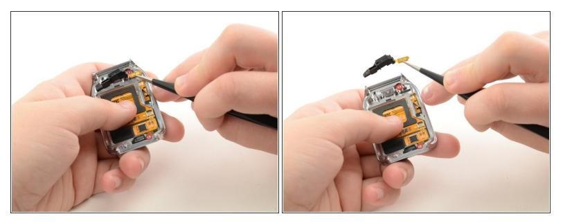
Use tweezers to grab the orange connector that is attached to side the home button assembly and lift to remove it from its adhesive.
