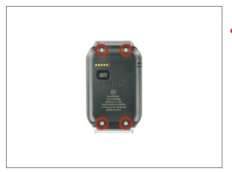
Remove the four 4.0 mm screws on the back of the Gear using a T5 Torx Screwdriver.
