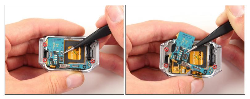
• Once the safety belt is removed, use tweezers to take the motherboard out of the Gear 2.
