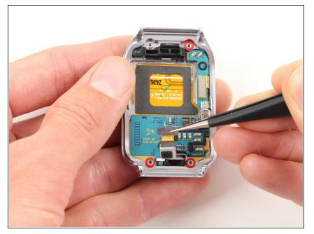
• Use tweezers to carefully lift the camera from its slot out of the case.
