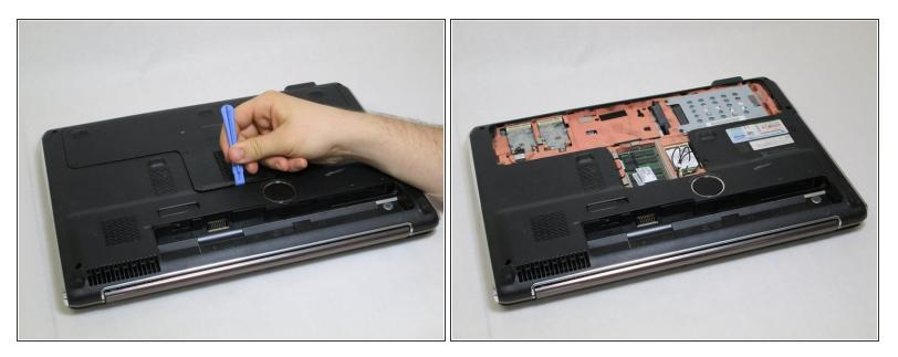
• Use the plastic opening tool to lift up the back plate and set it aside.
