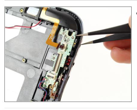
Once it is unscrewed, use the tweezer tool to pull the digital board straight out.
