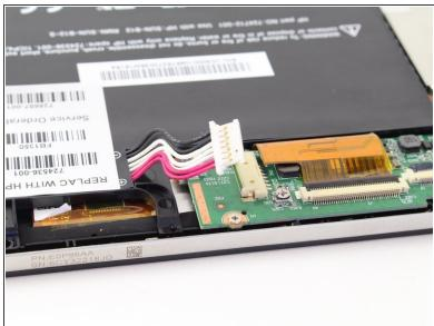
Push the white battery connector out of its housing using the pointed end of the spudger.
