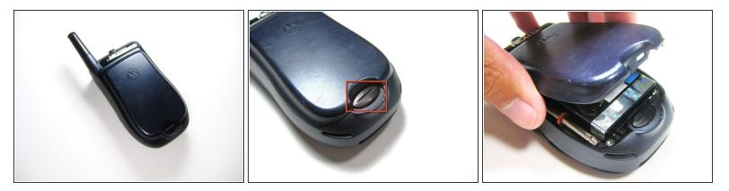
• Slide the notch downward while pulling the back cover off to remove it.
