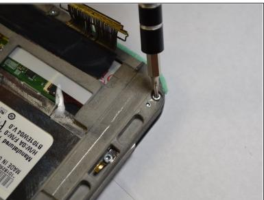
Using the T-6 Torx screwdriver, unscrew the 17 4mm screws along the edge of the screen frame.
