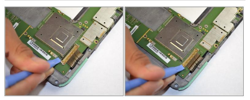
Using a plastic opener, lift the metal bar clasping the wire harness to the motherboard.
