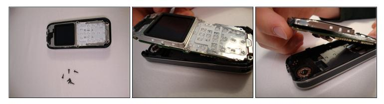
Lift the logic board and screen from the top.
