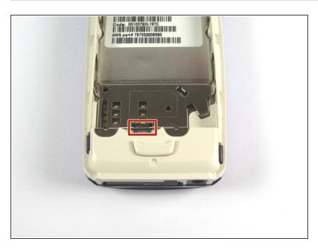
Gently pull back the small metal frame holding the SIM card into place, and lift open the frame.
