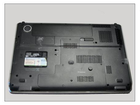
• Turn the device over so that the bottom side is facing up and the battery is facing away from you.
