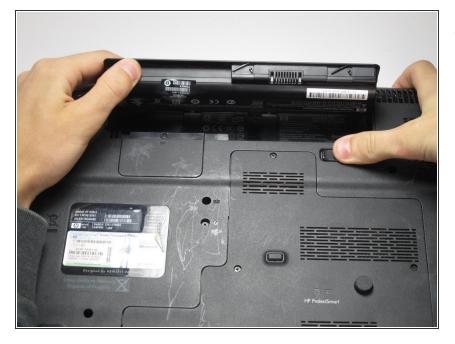
• With your thumb still holding the slider to the left, use the opposite hand to lift the battery out, removing it from the computer.
