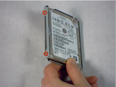
Remove the four silver 5 mm Phillips #1 screws from the hard drive.
