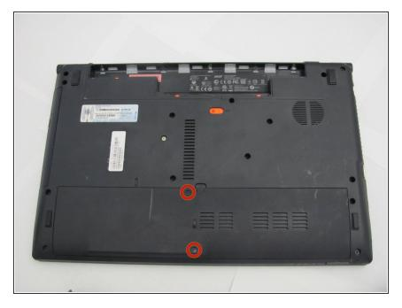
Locate and remove the two 5.3 mm
