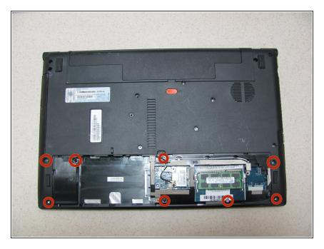
Remove the 8, 9 mm Phillips #1 screws holding the panel in place.
