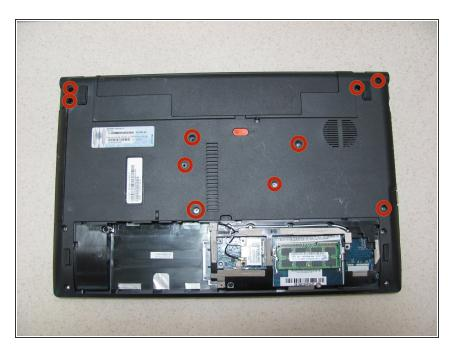
Flip the laptop and remove all 10 of the remaining 9mm screws from the back.
