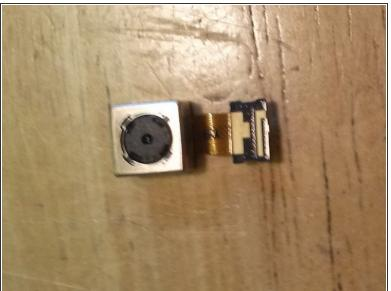
Use pry tool to disconnect camera cable and then remove the camera
