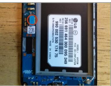
Use pry tool to disconnect 4 ribbon cables and two antenna wires.
