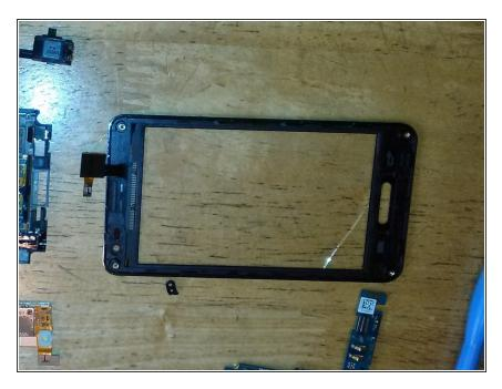
Use a heat gun or blow dryer to heat up the adhesive holding the glass in the frame. Carefully remove the glass using a pry tool.
