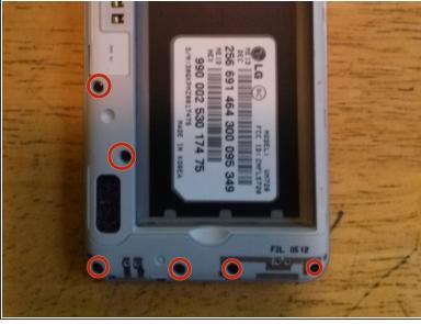
Remove 10 Philips Head screws
