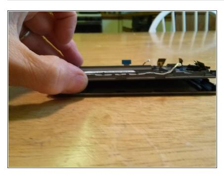
Use the pry tool to pry the front frame off of the main body of the phone.
