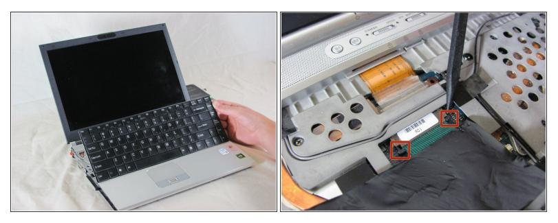
A The keyboard is still attached by ribbon cable, don't try to remove the keyboard entirely yet.
