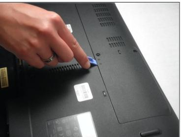
Once both screws have been removed use a plastic opening tool to lift the panel up.
