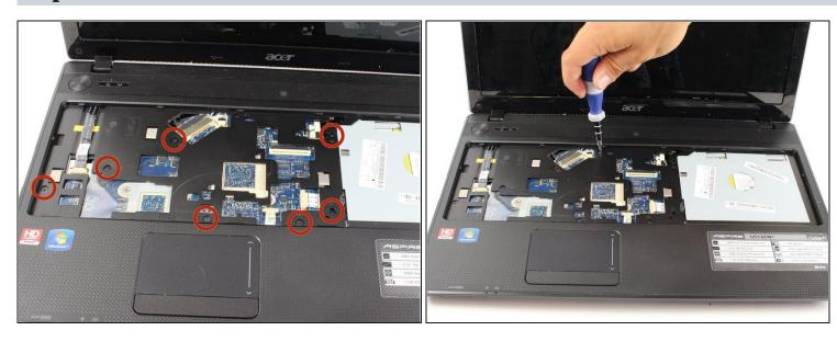
• Flip the Laptop back over, and unscrew the 1/4" diameter head 7/32" length screws indicated in the picture.
