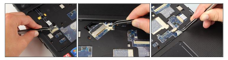
• Here is a close-up of all of the connectors. Remember to use tweezers on the black part and carefully pull out both sides. Once it has been moved back slightly, pull the connector out just like the keyboard.
