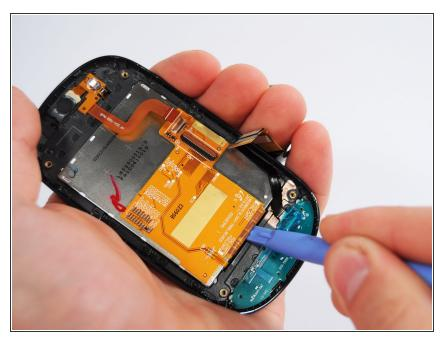
• Use a plastic opening tool on the bottom of the LCD to pry it off.
