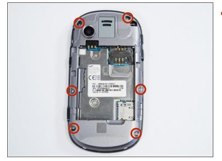
Remove the six 2.8 mm Phillips screws.
