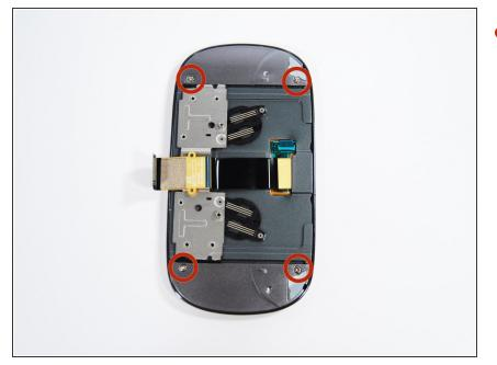
Remove the four 2.5 mm Phillips screws.
