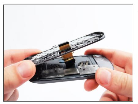
• Remove the keyboard housing from the screen housing.
