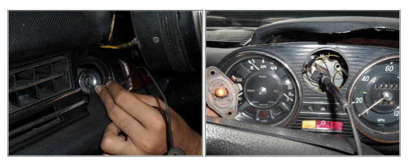
If the bulb lights up, the power supply to the clock is good.
