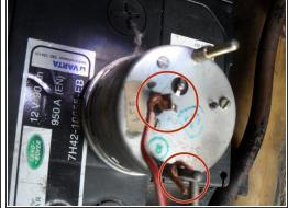
Connect the screw (located behind the clock) to the negative supply of the battery, and then the small pin to the positive supply.
