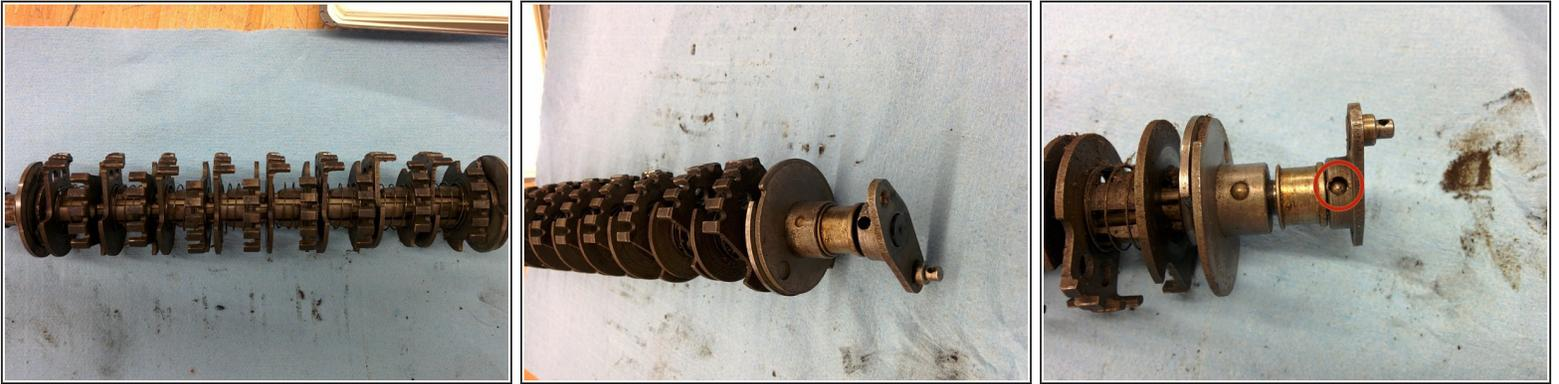
**i** It's called that because when you press a key, rock bars cause the plates on the assembly to move so that the same number of teeth as the key you pressed will be selected to engage other gears.
