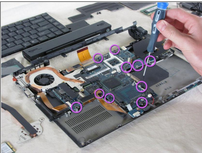
**⚠ Caution:** Ground yourself before removing the logic board. Static electricity can damage the logic board.
