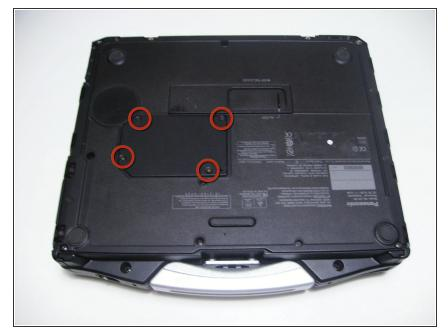
Use a Phillips size 0 screwdriver to remove the 4 screws holding down the ram cover.
