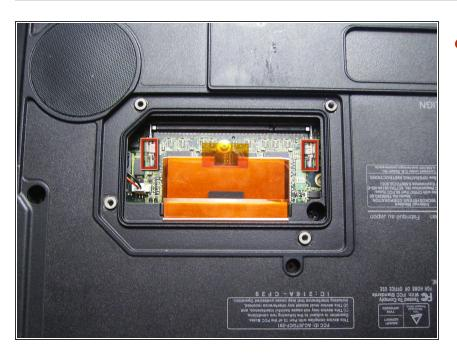
Pull the clips aside to release and remove the RAM.
