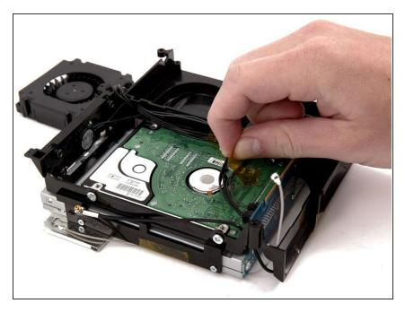
Peel up the yellow tape securing the speaker and fan cables to the bottom of the hard drive.
