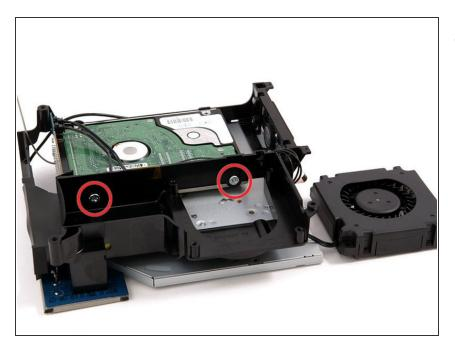
Use a #1 Phillips to remove the two screws attaching the right side of the hard drive to the plastic framework. You'll need to angle the screwdriver down to get access to the lower right screw. Be sure to apply steady force to the screws and turn slowly so as not to strip them.
