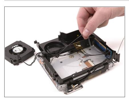
Deroute the speaker cable from the plastic framework, removing tape as necessary.
