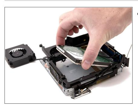
Lift the hard drive out of the assembly.
