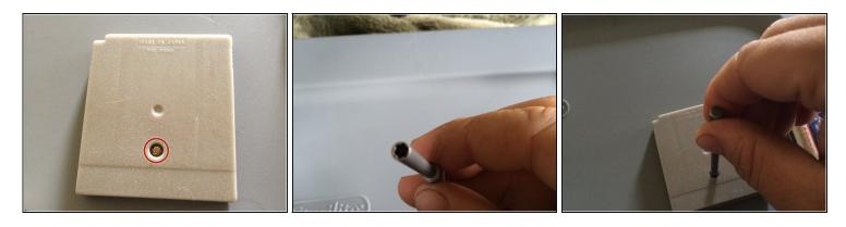
• On the back side of the cartridge is a priority security bit and you will have to remove it.
