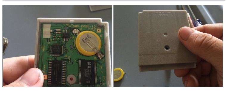
The final step is to set the board back into the plastic housing slide the cover shut and tighten the screw
