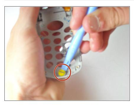
To remove the microphone, insert your opening tool under microphone and push upward to pry microphone away from the front cover.
