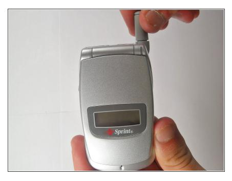
Hold antenna between your fingers and unscrew in a counterclockwise direction.
