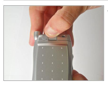
Use your thumb to pull the tab in an upward motion to release the battery.
