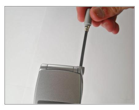
You will remove antenna by pulling it in an upward motion away from the socket.
