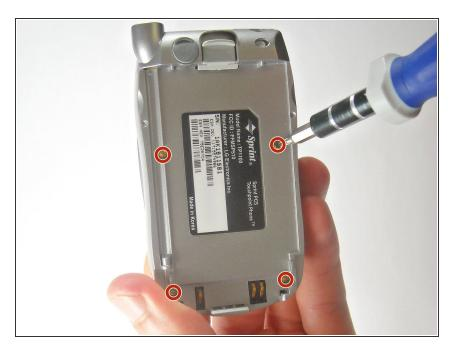
Use your screwdriver to unscrew the four screws from the back plate.
