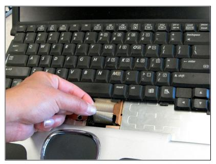
• Pull the cable and lift up to release.
