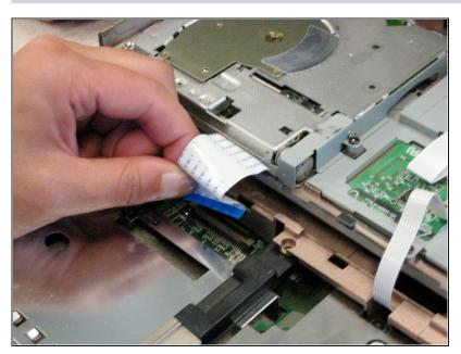
• <u>Disconnect the ribbon</u> <u>connector</u> from the socket.
