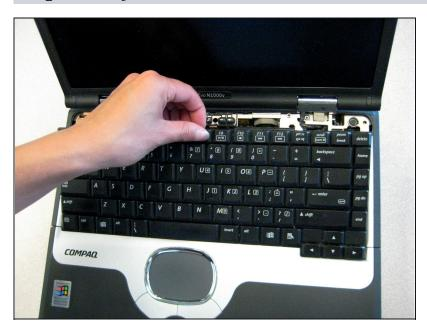
Lift the back edge of the keyboard and pull towards the screen.
