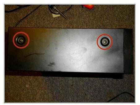
Turn the amplifier over onto its side and you will find two Phillips #2 screws holding the main black casing on, on each side of the amplifier. Remove them using the Phillips #2 screwdriver.
