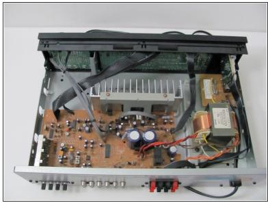
Slide off the case to expose the internal components of the receiver.
