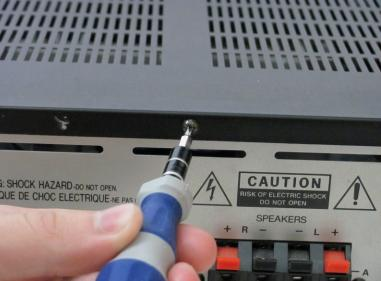
Remove the top screw on the back panel.
