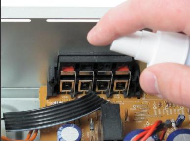
• Lightly spray the input and output connectors with DeoxIT on the inside of the back panel.
