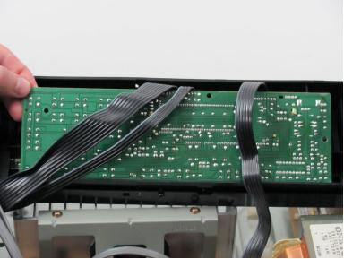
You will see the same snaps along the top of the logic board. Press the heads of the snaps down and pull the logic board out and up.
