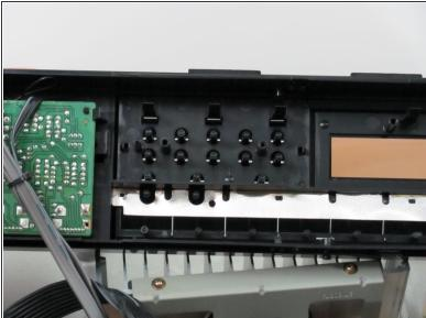
You will see that each button on the face plate has a button pin that presses the corresponding button on the logic board. Visually check if any of these pins are bent or broken.
