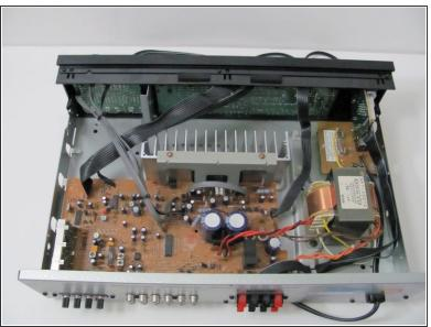
Slide off the case to expose the internal components of the receiver.
