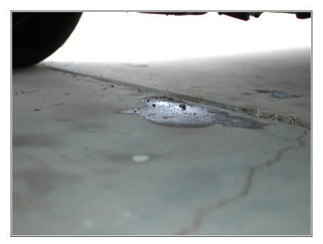
A power steering leak can be tricky to identify at at least initially.
