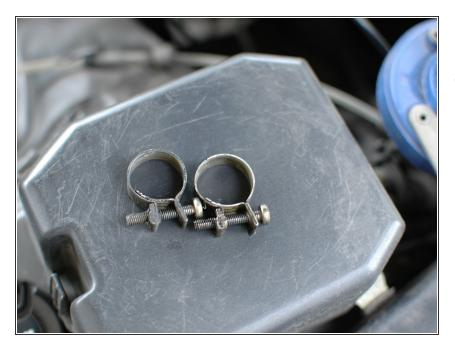
Inspect the hose clamps and clean or replace them as needed. These clamps were in good shape and were re-used.
